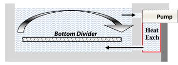
The discharge from the heater exchange is directed under the bottom divider of the tank. A much larger volume of liquid gets drawn down under the false bottom through a slot at one end. This flow mixes with the heat exchanger discharge. As it emerges from under the bottom divider, the liquid is so close to the mean tank temperature, that **gradients are less than 0.002** °C throughout the bath.
