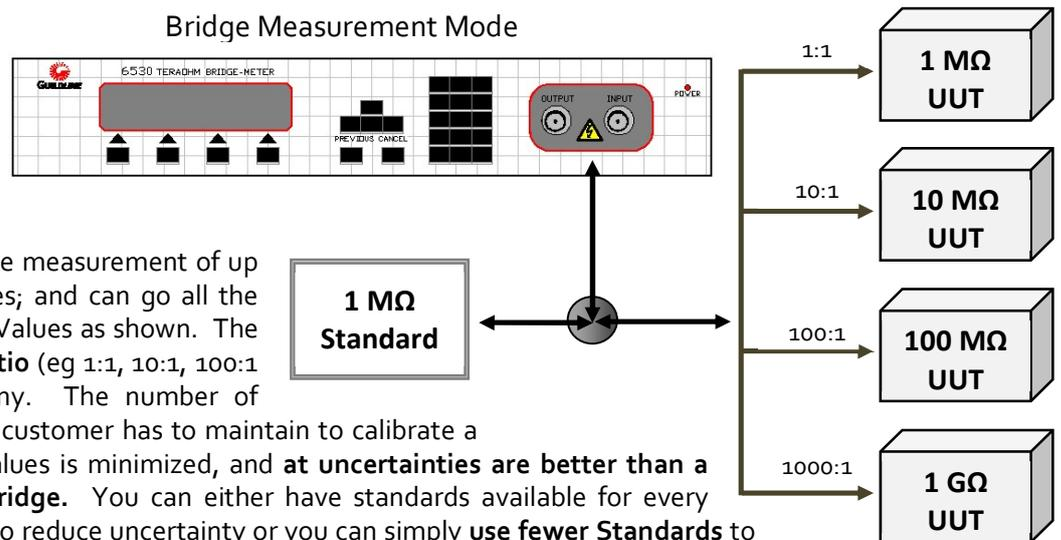
This process is **completely automated with the TeraCal software** that is provided. Add a 6564 Scanner, and now you are talking about **true automation** and the cross-verification of results. In contrast a **dual source bridge does not have this flexibility**.
