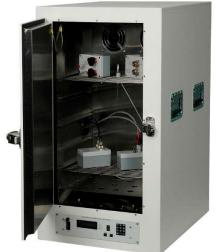
Like the 6530, this **Air Bath is fully programmable** via the Standard **IEEE 488.2 bus** with optional drivers already in the TeraCal<sup>™</sup> Software or **you can program this Air Bath** right from the **front panel** with a full menu system!
