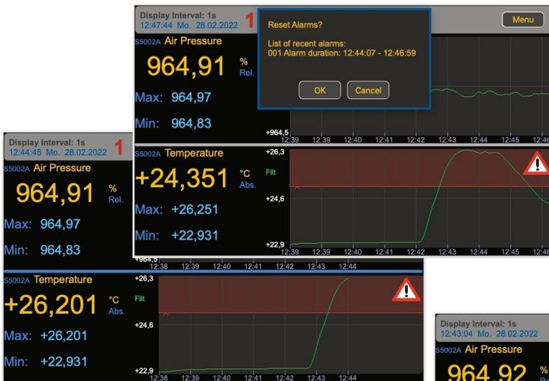
At the left side you can see how the measured temperature exceeds the limit value. Conact #1 is activated and an exclamation sign is being displayed.
